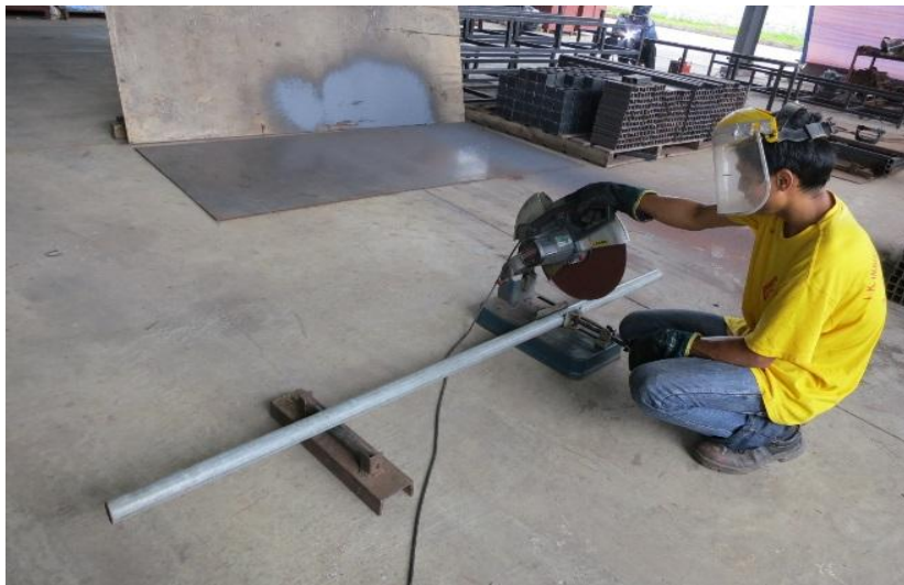
Cutting / resize of damage pipe
