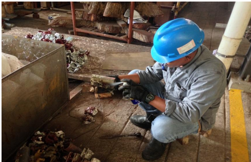
Lubricating / greasing of coupling
